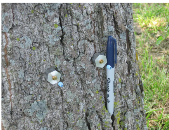
Figure 4.7. In-planta sampler and SPME device during sampling at Kellwood Site.
